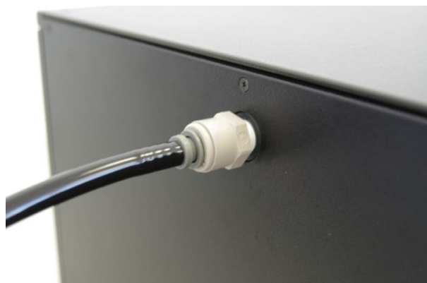
Figure 4. Fit the inlet connector on the rear panel of the Aethalometer and connect the sampling line tubing to it.
