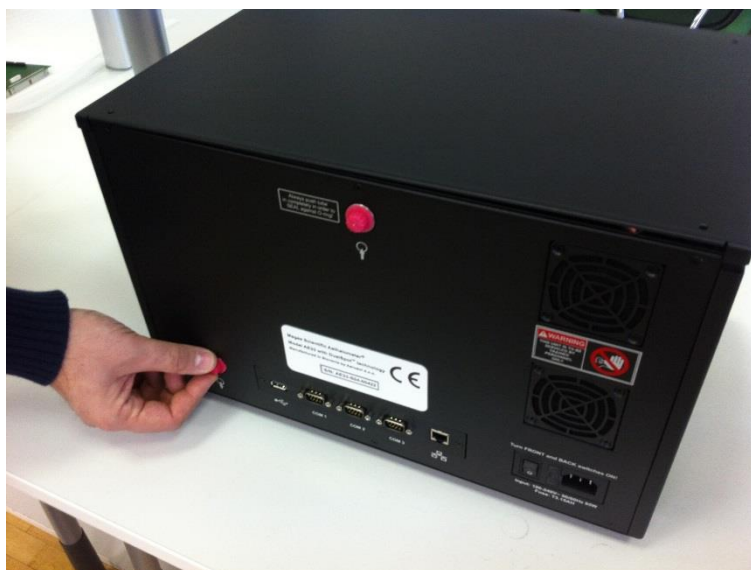
Figure 3. Remove the red protective caps on the rear panel of the instrument before switching it on!
