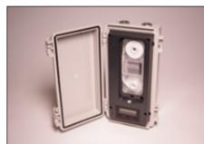
The microAeth® MA350 is a real-time 5-wavelength UV-VIS-IR Black Carbon monitor housed in an outdoorrated case with an 85 sampling location automatic filter tape advance system which allows for 3-12 months of continuous measurements.
